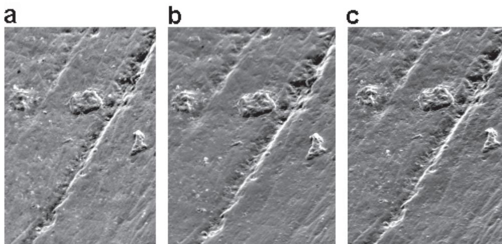
FIGURE 5. Three images of the same enamel surfaces obtained with the original teeth (a), the Epo Tek #301 cast (b), and the Feropur PR-55 cast (c). All images were obtained at 500 $\times$  magnification.
