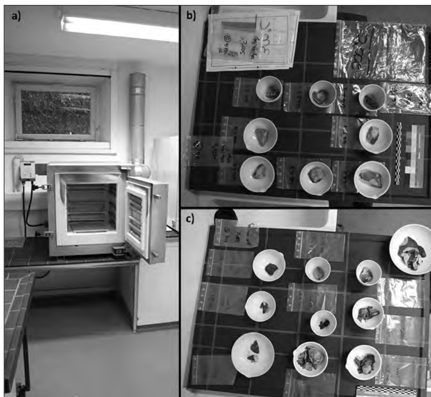
FIGURE 8: Heating procedure. a) Muffle kiln used for the controlled experiments, b) one series of pieces before heating, c) another series after heating, in the bigger heating bowl there are the pieces distributed into the kiln. Illustration by J. A. Frick.
